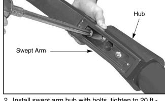
2. Install swept arm hub with bolts, tighten to 20 ft.-lbs.
