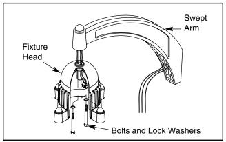
Install bolts and lock washers through fixture head as shown. Pull wires through arm and out arm access cover. IMPORTANT: Keep wire tight when attaching fixture to arm to avoid pinching wires.
