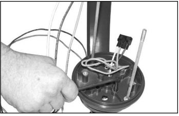
Install the fixturebase to down cast arm. Important!
