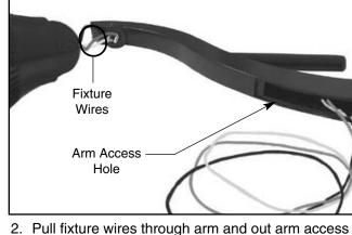
Pull fixture wires through arm and out arm access hole. IMPORTANT! Keep wires tight when attaching fixture to arm to avoid pinching wires.
