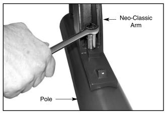
4. Install neo-classic arm to pole with bolts, tighten to 20-ft. lbs.
