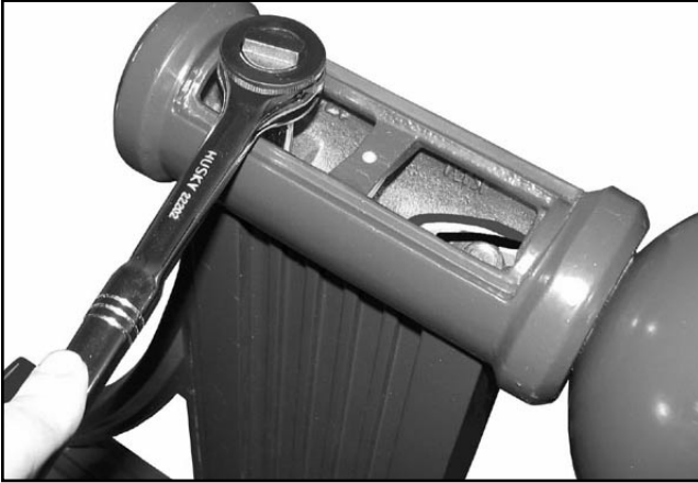
5. Install arm fitter with fixture head to ribbon arm. Tighten to 20-ft. lbs.
