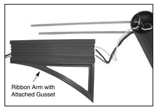
3. Hold pole backing plate inside pole & thread draw bolts into backing plate. Slide ribbon arm over draw bolts pulling wires tight so they do not get pinched. Note: Arm will have a circular cut to fit a round pole.
