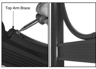
Attach top brace to ribbon arm. Tighten nuts on rods to 20 ft.-lbs. tighten brace hardware securely.
