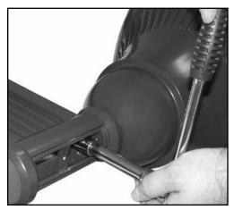
5. Install arm fitter with fixture head to ribbon arm loosely. Connect fixture wires to field wires observing polarity, i.e.; green-to-ground, white-to-common, and black-to-voltage. (See fixture installation instructions.)
