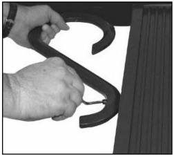
Install top scroll to ribbon arm and pole. Torque nuts on rods to 20 ft.lbs. Tighten scroll hardware securely.
