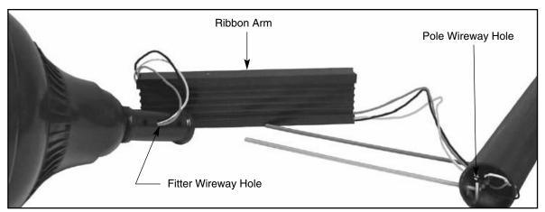
4. Hold pole backing plate inside pole & thread draw bolts into backing plate. Slide ribbon arm over rods pulling wires tight so they do not get pinched. **Note:** Arm will have a circular cut end to fit a round pole.
