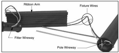
3. Hold pole backing plate inside pole & thread draw bolts into backing plate. Slide ribbon arm over draw bolts pulling wires tight to they do not get pinched. **Note:** Arm will have a circular cut end to fit a round pole. (See fixture installation instructions for fixture attachment.)
