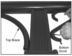
Attach top brace and bottom scroll, torque nuts on arm rods to 20 ft.-lbs. Tighten other fasteners securely.
