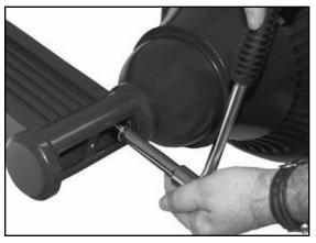
5. Slide ribbon arm over rods pulling wires tight so they do not get pinched. Attach arm fitter to ribbon arm loosely.
