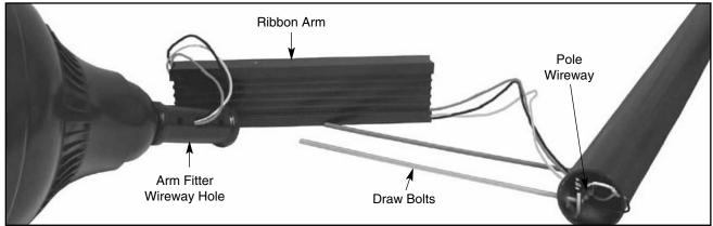
4. Hold pole backing plate inside pole & thread draw bolts into plate. Thread wires through wireway hole in arm fitter then through ribbon arm and wireway hole in pole. Slide ribbon arm over draw bolts pulling wires tight so they do not get pinched. Note: Arm will have a circular cut end to fit a round pole. Connect wires at pole hand hole observing polarity, i.e.; green-to-ground, white-to-common and black-to-voltage.
