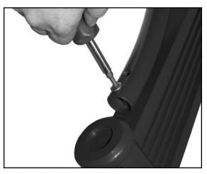
6. Attach top brace to ribbon arm and pole. Tighten nuts on rods to 20 ft.-lbs. Tighten brace hard-ware securely.
