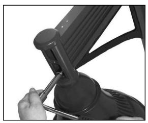
5. Slide ribbon arm over rods pulling wires tight so they do not get pinched. Attach arm fitter to ribbon arm loosely.
