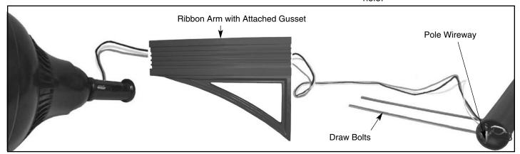
4. Hold pole backing plate inside pole & thread draw bolts into backing plate. Slide ribbon arm over draw bolts pulling wires tight so they do not get pinched. **Note:** Arm will have a circular cut end to fit a round pole. Connect fixture wires to field wires at pole hand hole, observing polarity, i.e.; green-to-ground, white-to-common and black-to-voltage.
