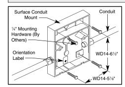
Attach surface conduit mount to existing surface with hardware (by others) of adequate strength for installation requirements. Attach conduit per required application. Use proper sealant all around conduit fittings and mounting hardware.
