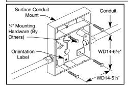
Attach surface conduit mount to existing surface with hardware (by others) \of adequate strength for installation requirements. Attach conduit per required application. Use proper sealant all around conduit fittings and mounting hardware.
