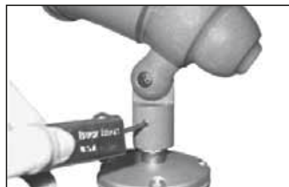
5. Loosen set screw, adjust fixture rotation, and tighten set screw.
