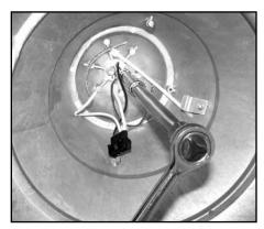
Install fixture head onto swept cast arm. <u>IMPORTANT!</u> Keep wires tight when attaching fixture to swept cast arm to avoid pinching wires. Connect fixture wires to supply wires observing polarity, i.e.; green-to-ground, white-tocommon, and black-to-voltage. (See fixture installation instructions.)
