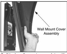
5. Attach wall mount cover plate with arm and fixture head attached, to wall plate with two (2)  $\frac{5}{16}$ -18 x 1  $\frac{1}{4}$ " socket head cap screws.
