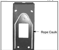
Remove wiring inspection cover from wall mount cover and wall mount cover plate. Adhere rope caulk in a continuous strip into the wall plate groove. Allow mastic to extend well above the wall plate surface to ensure a proper seal.
