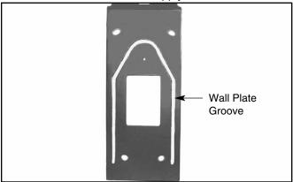
Remove wiring inspection cover from wall plate and wall mount cover plate. Adhere rope caulk in a continuous strip into the wall plate groove. Allow caulk to extend well above the wall plate surface to ensure a proper seal.
