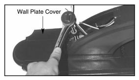
4. Attach arm to wall mount plate cover using two (2) 5/16-18 x 11/4" hex head cap screws (supplied).
