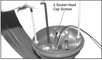
3. Attach fixture base to S-Shaped Down Cast Arm using four (4) socket head cap screws. Tighten securely. **IMPORTANT! Keep wires tight when attaching fixture to down cast arm to avoid pinching wires.** (See fixture installation instructions for fixture attachment.)
