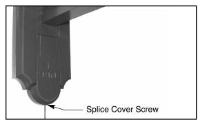
10. Attach splice cover using the 10-32 flat head stainless steel socket screw.
