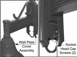
Attach wall plate cover assembly to wall plate. Secure using two (2) socket head cap screws. Connect fixture wires to supply wires observing polarity, i.e.; greento-ground, white-to-common, and black-tovoltage.
