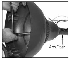
4. Attach fixture to arm fitter. (See fixture installation instructions.)
