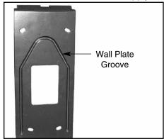
Remove wiring inspection cover from wall plate and wall mount cover plate. Adhere rope caulk in a continuous strip into the wall plate groove. Allow caulk to extend well above the wall plate surface to ensure a proper seal.
