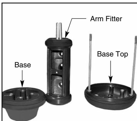
5. Attach base & base top to arm fitter using (4) socket head cap screws. Tighten securely. **IMPORTANT! Keep wires tight when attaching fixture to avoid pinching wires.**
