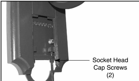
8. Attach wall plate cover assembly to wall plate. Secure with two (2) socket head cap screws. Connect wires observing polarity, i.e.; green-to-ground, white-to-common, and black-to-voltage.
