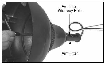
4. Install fixture to arm fitter. Thread fixture wires through arm fitter and out wire way hole.
