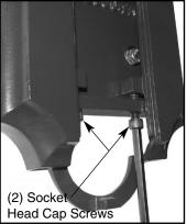
Attach wall mount cover with arm assembly to wall plate using two (2) socket head cap screws. Connect fixture wires to supply wires observing polarity, i.e.; green-to-ground, white-to-common, and blackto-voltage. (See fixture installation instructions.)
