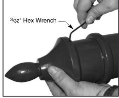
6. Attach finial to pole cap base using a <sup>3</sup>/<sub>32</sub>" hex wrench.
