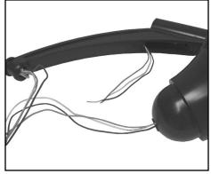
Pull wire through arm and out arm access cover.
