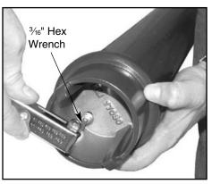
5. Attach pole cap base to pole top using a 3/16" hex wrench.
