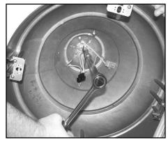
Install fixture head to side pole swept cast arm with washers & nuts, tighten to 20 ft.-lbs.
