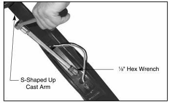
Attach up cast arm to pole with bolts, tighten to 20 ft.lbs. All mounting hardware is supplied by Kim Lighting.
