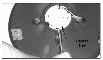
4. Join wiring quick-disconnect and install ballast tray through keyholes onto screws; tighten securely.
