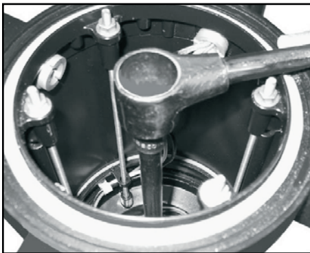
5. Tighten securely using 3/16" socket, 12" extension and ratchet.
