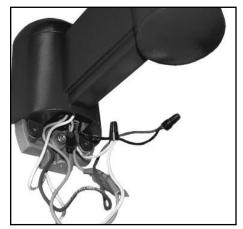
Mount fixture over wall mount plate. Connect fixture wires to supply wires observing polarity, i.e.; green-to-ground, white-tocommon, and black-to-voltage.
