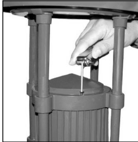
6. Remove ballast cover from fixture using a hex wrench.
