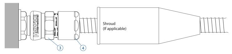
If enclosure end of middlenut is exposed, pull down deluge boot to cover the exposed end.
