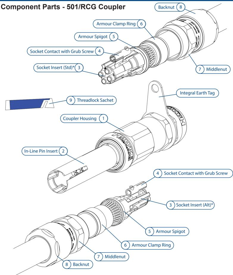
\* Supplied socket inserts are coloured black (standard) or natural (alternative). Parts are dimensionally identical but the pin numbering is inverted to ensure correct through numbering.
