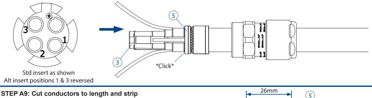
Cut conductor to 26mm from top of spigot. Use the groove indicator in the insert as a visual aid. The conductor should not extend past this cut line. Strip conductor back past the insert shoulder which indicates the strip line.
