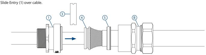
Note: A spare entry component could be used to clamp the armourings, which removes the need to remove the inner seal of the gland to be assembled.
