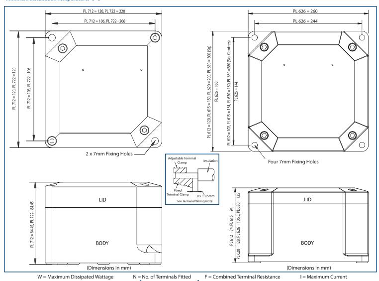
$W = N \times F \times I^{\uparrow}$   $N = W / F \times I^{\uparrow}$   $I = Sqrt (W / N \times F)$ **Note:** Combined Terminal Resistance = Resistance of Maximum Conductor Length (see BS 6360 and table below) + Terminal Resistance
