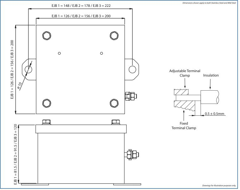
W = Maximum Dissipated Wattage N = No. of Terminals Fitted F = Combined Terminal Resistance I = Maximum Current  $W = N x F x I^2$  N = W / F x I<sup>2</sup> I = Sqrt (W / N x F)
