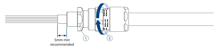
**NOTE:** Support the cable to prevent it twisting. To aid wiring inside the enclosure, it may be beneficial to strip the inner sheath as shown above.
