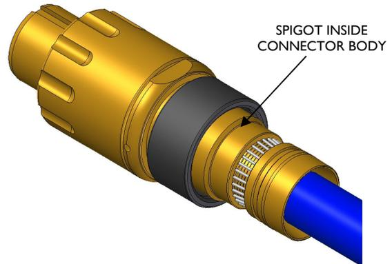
20) Slide the middle nut over the clamp / spigot and hand tighten onto the connector body, then further tighten 1/2 to 3/4 of a turn with a spanner while holding the front shell with a spanner
