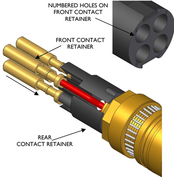
18) Slide the front contact retainer over the contacts and snap into place with the rear contact retainer. Push the clips of the rear contact retainer firmly down to ensure they are not protruding (will only fit in the correct orientation).
