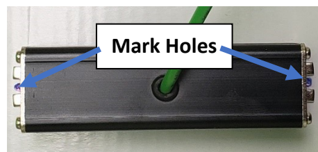
Figure 12 - Mark for Pilot Holes
