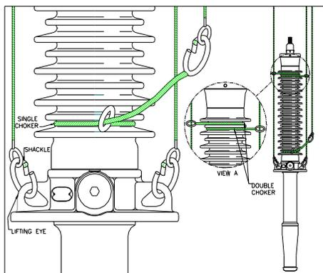
Lift the bushing by raising both crane hooks simultaneously maintaining the air end of the bushing slightly above the oil end until ready to lower the oil end of the bushing.
