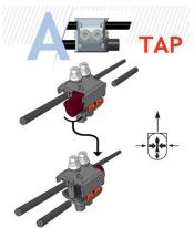
Remove the main cap and adjust the position of the tap seal cap as needed.
