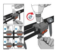
Utilize either an impact wrench or a hex socket wrench for manual connector tightening. Alternate tightening as demonstrated in the image.
