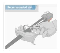
Secure the tap cable by using a plastic tie.
