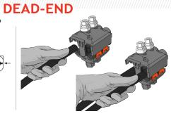
Ensure the cables are fully inserted into the caps, continuing until it reaches a stop.
