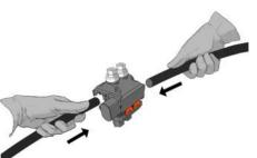
Ensure the cables are fully inserted into the caps, continuing until it reaches a stop.
