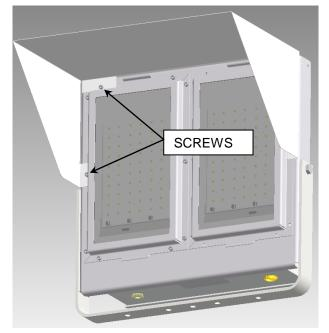
To install lens assembly guard, verify that the luminaire is completely assembled. Install lens guard on lens assembly by hooking the guard's end tabs under the luminaire housing's end tabs. Verify a tight attachment.
