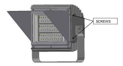
To install lens assembly guard, verify that the luminaire is completely assembled. Install lens guard on lens assembly by hooking the guard's end tabs under the luminaire housing's end tabs. Verify a tight attachment.
