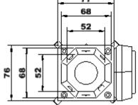
Spigot Entry for Post Top Mounting suitable for Poles with Outside Diameters 40 - 55mm
