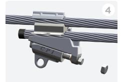
Using a 3/4 or 9/16 socket, tighten the outer bolt until it shears.
