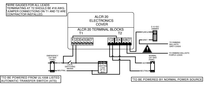
If Class 2 circuit, use knockout provided on enclosure and separate conduit to route these wires (see Note in Step 4 on Page 2).
