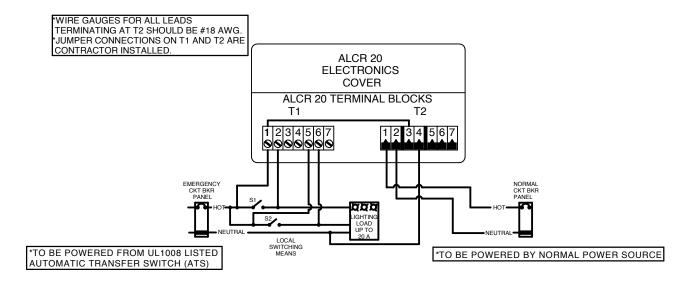
\*NOTE: WIRE GUAGES FOR ALL LEADS TERMINATING AT T2 SHOULD BE #18 AWG. CONNECTED LIGHTING LOAD. **GROUND UNIT USING SUPPLIED GREEN LEAD WIRE.** JUMPERS FROM T1 TO T2 MUST BE INSTALLED BY CONTRACTOR
