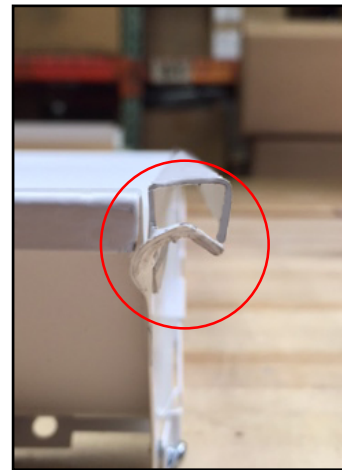
Figure 3. Hinge Front View (Incorrectly Aligned)
