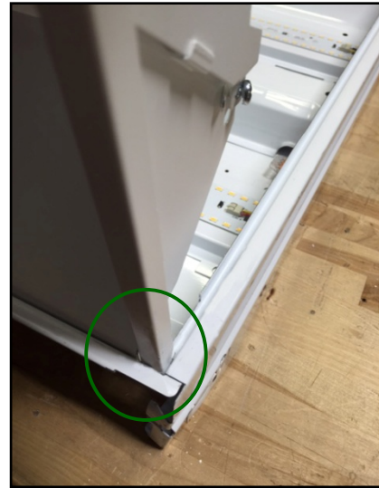
Figure 7. Hinges slid backwards towards side of housing.
