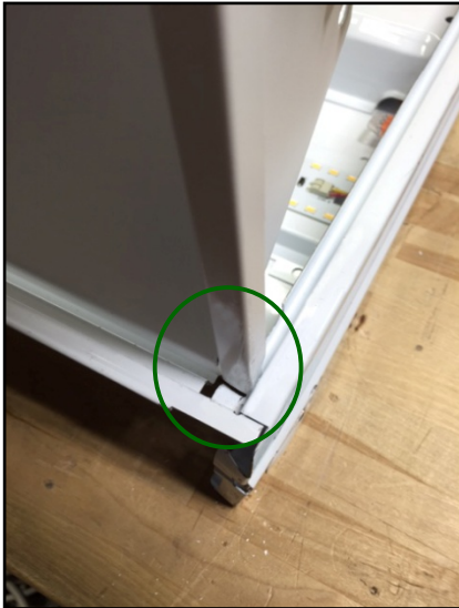
Figure 6. Connection of the right hinge to the housing.
