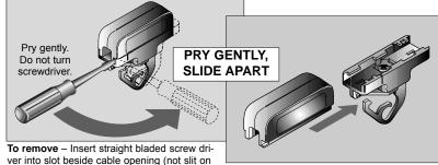
side of trolley) and pry gently as shown above. Do not turn screwdriver. Slide Apart.
