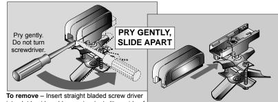
into slot beside cable opening (not slit on side of trolley) and pry gently as shown above. Do not turn screwdriver. Slide Apart
