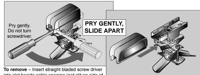
into slot beside cable opening (not slit on side of trolley) and pry gently as shown above. Do not turn screwdriver . Slide Apart
