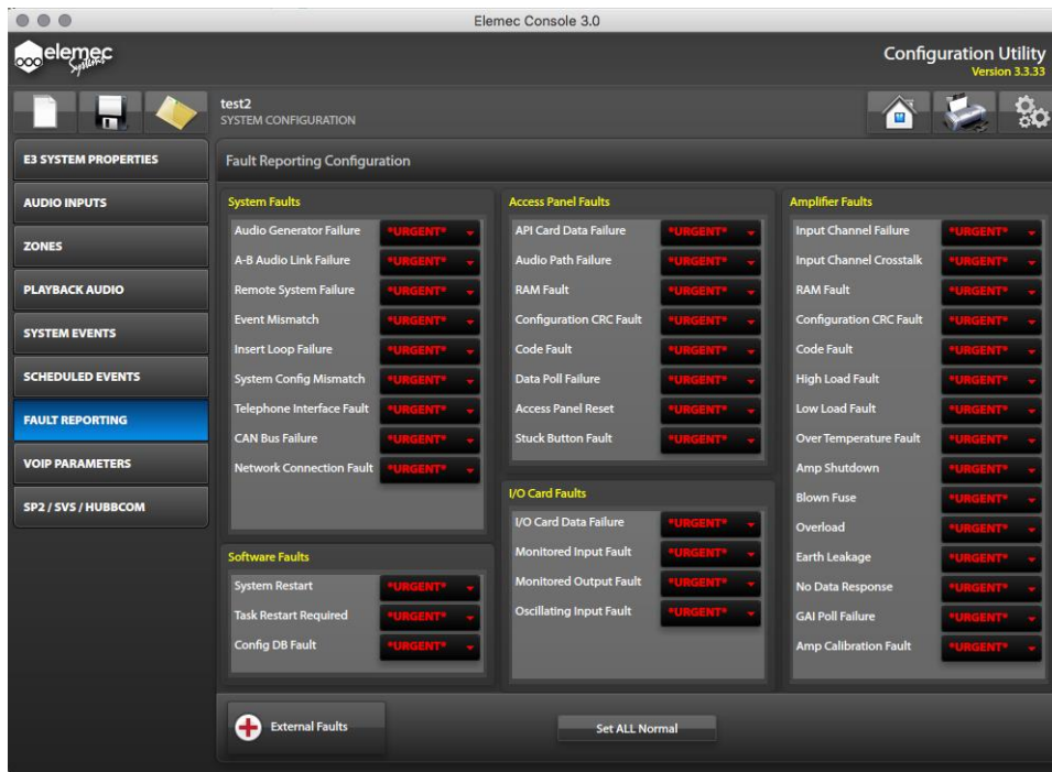
Figure 94. Fault Reporting Configuration
