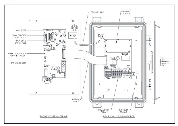
Figure 3. SP2 Fiber Weatherproof Station—Interior View
