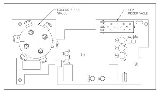
Figure 9. Fiber Termination PCBA
