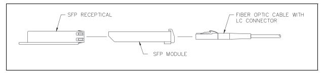
Figure 10. SFP Transceiver Insertion and Fiber Plug-in
