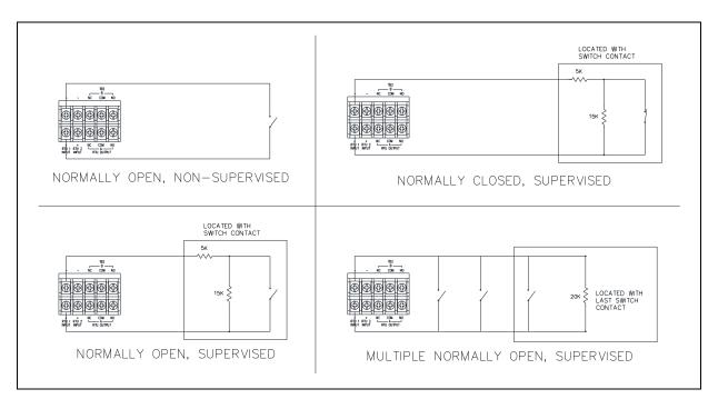
Figure 6. RTU Input Wiring Configurations for Cable Monitoring
