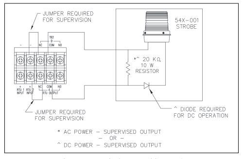
Figure 7. Supervised Output Wiring—TB2
