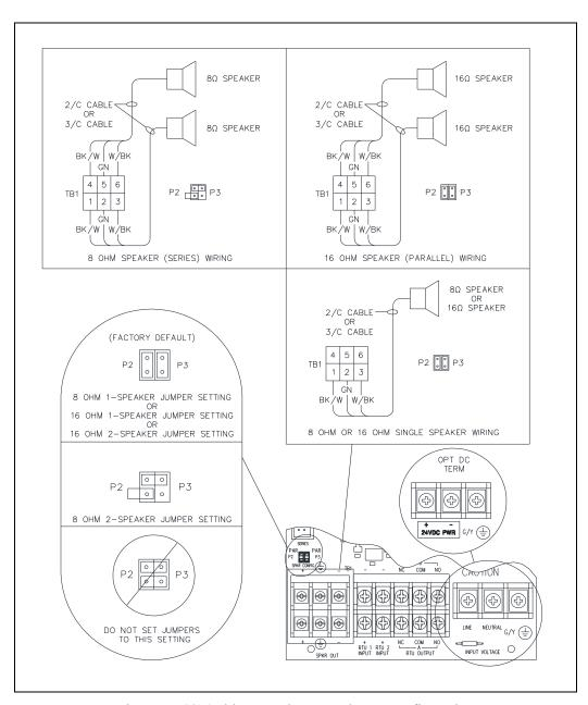
Figure 5. 8/16-ohhm Speaker Impedance Configuration and AC/DC Termination at TB3
