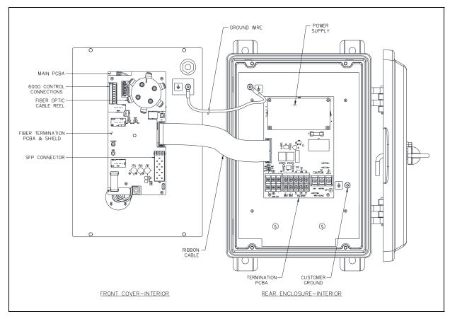
Figure 11. SP2 Fiber Weatherproof Station—Interior View
