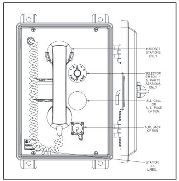
Figure 1. SP2 Station Front Panel
