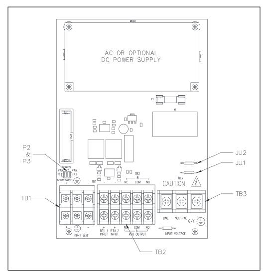
Figure 4. SP2 Standard Termination PCBA
