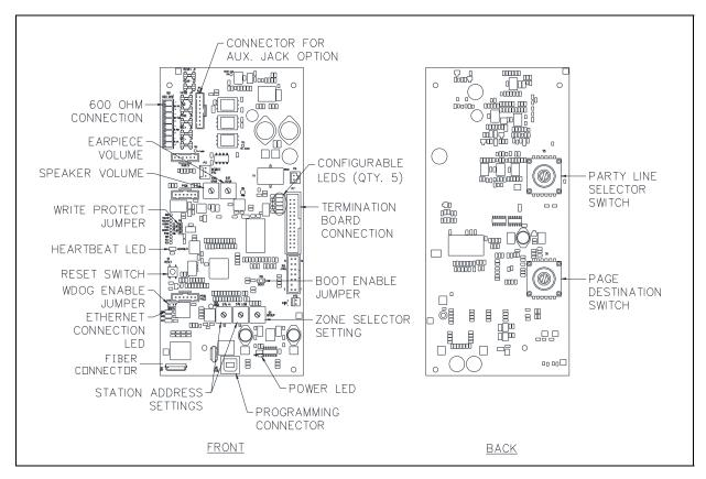
Figure 12. Main PCBA (Front and Rear Views)
