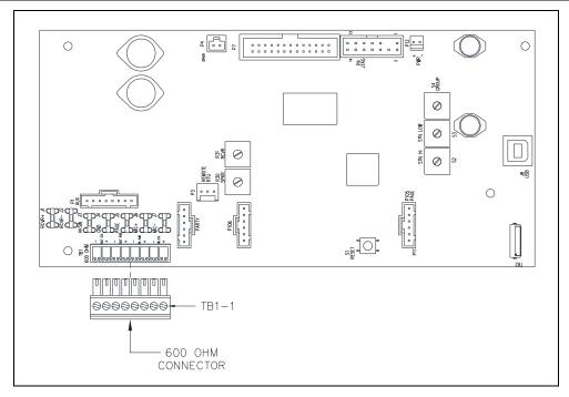
Figure 8. SP2 Main PCBA (Fiber)
