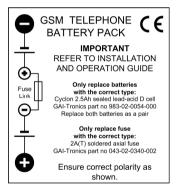
Always ensure the batteries are connected before connecting the power supply, or the batteries may not charge.
