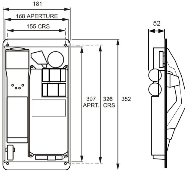
Titan telephones supplied for flush mounting have a slightly different faceplate to those supplied with a rear enclosure – in particular the fixing holes are in different positions and there are no corner cut-outs (for door hinges). These models are usually described as “Titan fp” and the supplied mounting kit contains round-headed screws and no glands.
