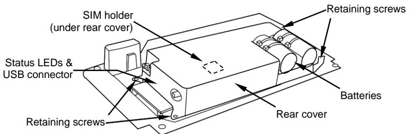
To remove the rear cover, remove the 4 retaining screws and carefully lift it away from the PCB. Take care not to pull or strain the battery cable which connects between the rear cover and the PCB.
