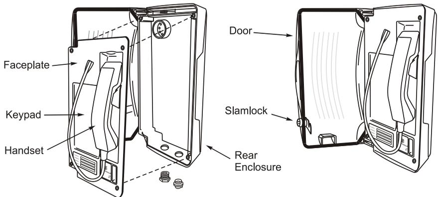
Most Titans are equipped with a heavy-duty spring-loaded door, but models are available with a soft-close door, without door and also as faceplate only, for flush mounting.
