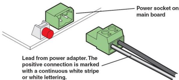
Power requirement is 9-18V dc, 3.6W. The telephone can be connected directly to a solar panel without the need for a charge controller.
