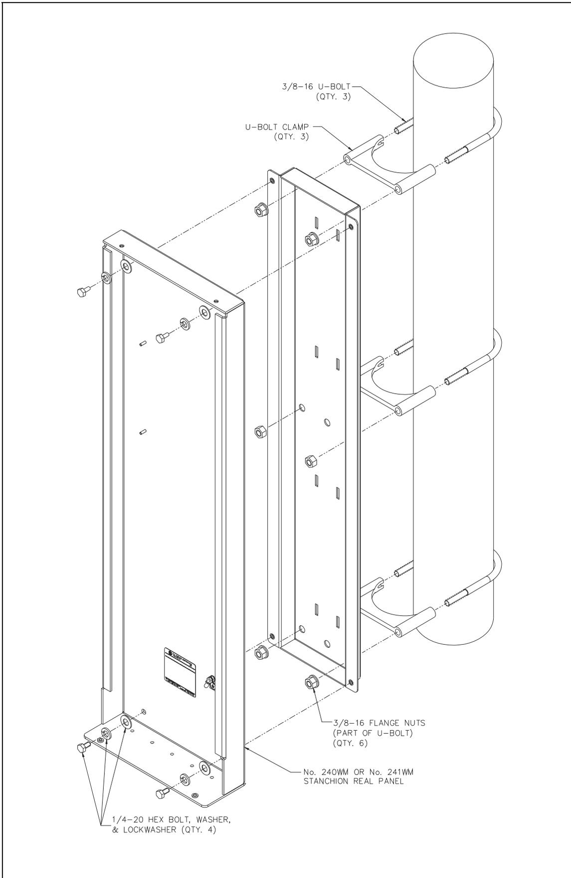
Figure 2. Bracket and Enclosure Installation
