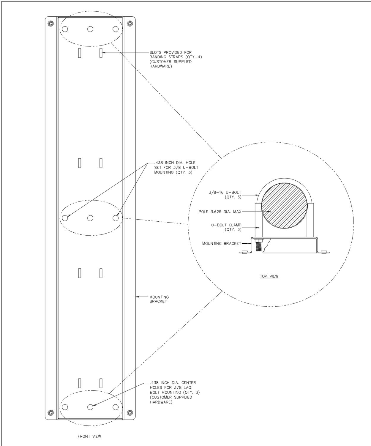
Figure 1. Pole Mounting Bracket Installation Detail
