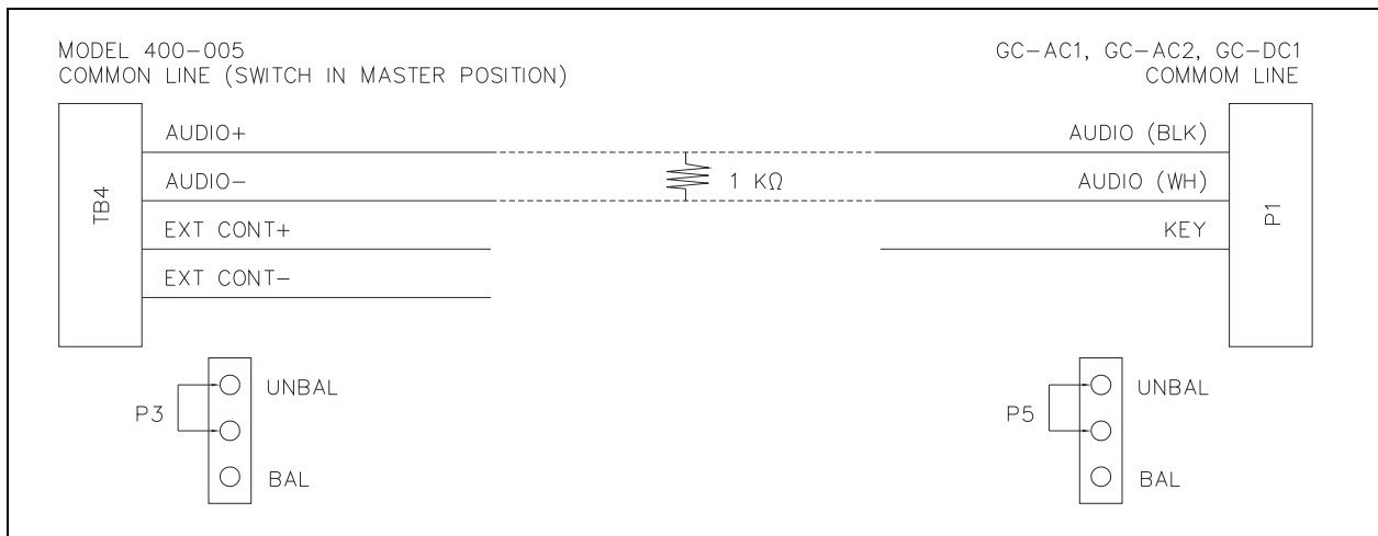
Figure 12. Unbalanced Common Line Configuration
