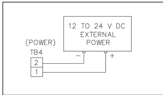
Figure 3. Power connections at TB4
