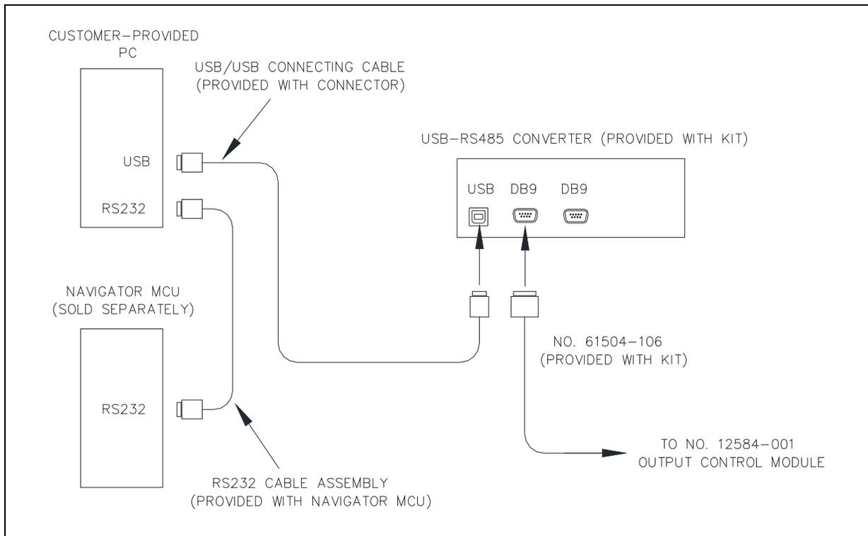
Figure 1. Typical Installation Block Diagram
