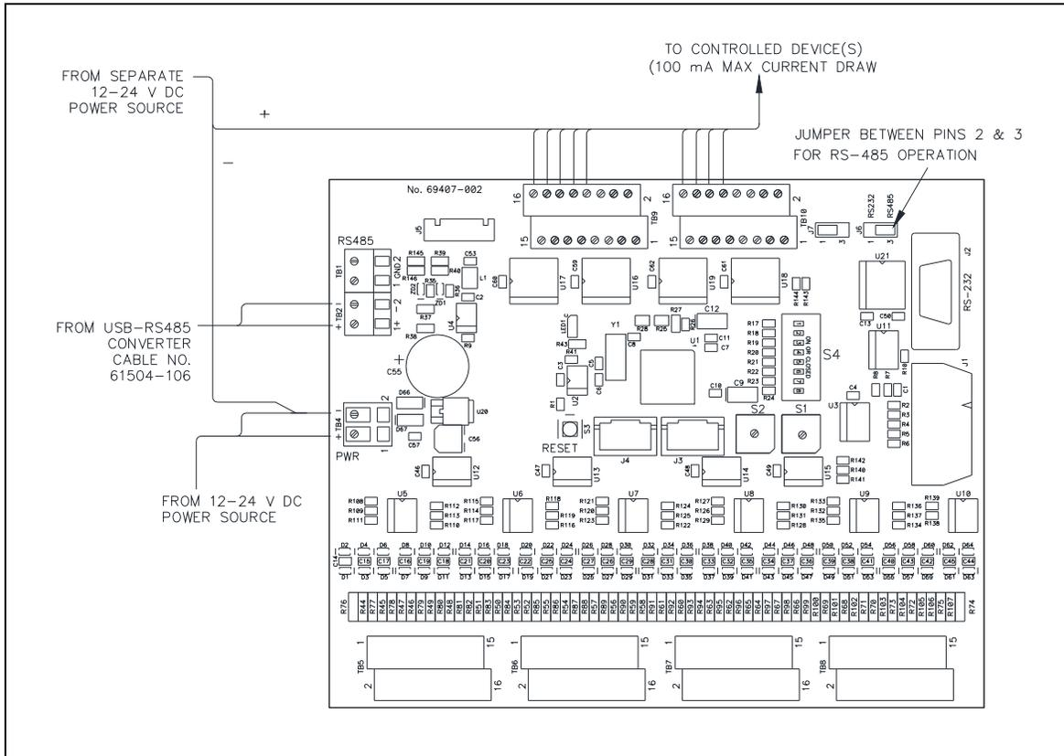
Figure 2. Model 12584-001 Output Control Module
