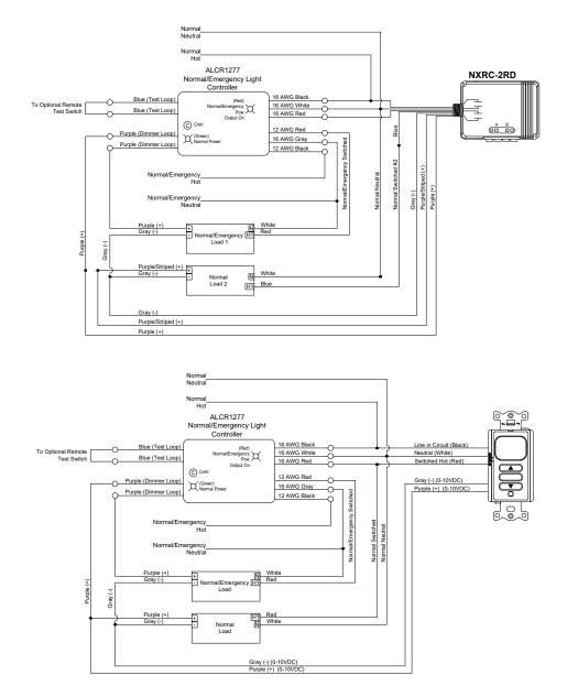
Caution: Prior to making any connections, verify that none of the loads are shorted. Failure to do so may result in personnel injury, damage to the unit, and void its warranty.
